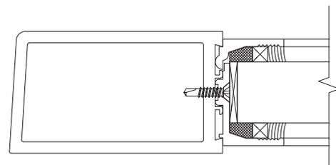
Note: Details show open for 1" large missile impact glazing. Option for 9/16" large impact missile glazing also available.
